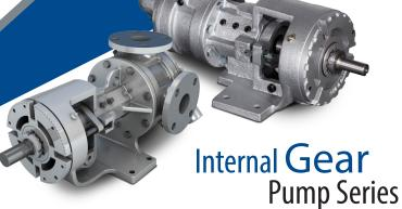
**G Series** pumps are available in cast iron and stainless steel with many features and options, including an enlarged bearing housing at the rear end of the pump that provides easy drive-end access to the shaft seal and single-point end-clearance adjustment. The pump casing also revolves to allow for multiple inlet and outlet positioning.
